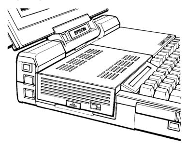
The TYPE indicator on the left side identifies the type of hard disk drive. You use this TYPE for the SETUP program. A 20MB hard disk is TYPE 2; a 40MB hard disk is TYPE 17.
